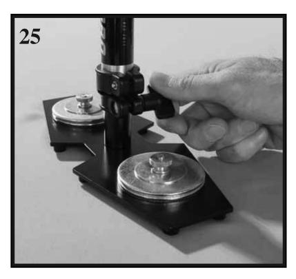
**Securely** tighten the "Adjustment Knob" on the TELESCOPING CLAMP by rotating the Knob clockwise as shown in this photo.
