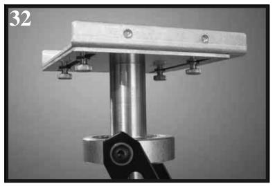
At this point you should have four BRASS THUMB SCREWS securing the MID PLATE to the BOTTOM PLATE.
