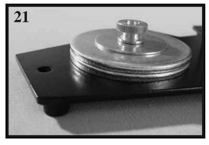
Secure the COUNTER WEIGHT DISKS with the BRASS THUMB NUTS as shown in this photo and repeat this procedure for the COUNTER WEIGHT DISKS on the other side of the BASE PLATFORM.
