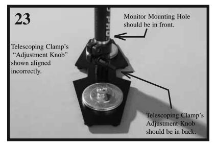
Now, insert the TELESCOPING POST with the attached BASE PLATFORM Assembly up and into the CENTRAL POST (the Central Post can be seen in photo # 2).
