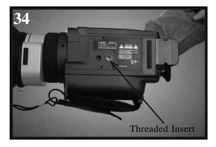
First, find the "Threaded Insert" on the bottom of your Camera.
