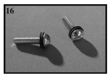
Now find a pair of bolts (example: 1/4" x 20 x 1") and attach RUBBER WASHERS as shown in the photo to the left.
