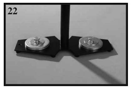
Both COUNTER WEIGHT DISK stacks should now be secured in place with the FENDER WASHERS and BRASS THUMB NUTS as shown in this photo.
