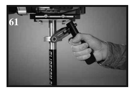
Do not allow the Handle of the Glidecam 2000 Pro to come in contact with the BOTTOM PLATE as in Photo # 61. If the Handle comes into contact with the BOTTOM PLATE it will limit your range of motion, and will result in "jerky", and unpleasant footage. Instead position the Handle as shown in Photo # 50.
