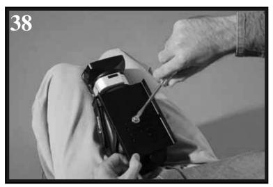
Make sure the HEAD PLATE is in alignment and square with the bottom of the your Camera, and make sure the "Threaded Insert" on the base of your Camera is aligned with one of the "Mounting Holes" in the HEAD PLATE.
