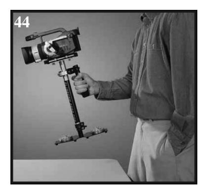
When testing for correct horizontal balance you need to make sure that you pick up your 2000 Pro from a flat and level surface (a table for example) and that you let the 2000 Pro hang freely as you hold it as shown in Photo #43. If the 2000 Pro is balanced correctly on its horizontal axis, then it will be level and upright, with the CENTRAL POST in a virtually perfect vertical position, as pictured in photo #43.
